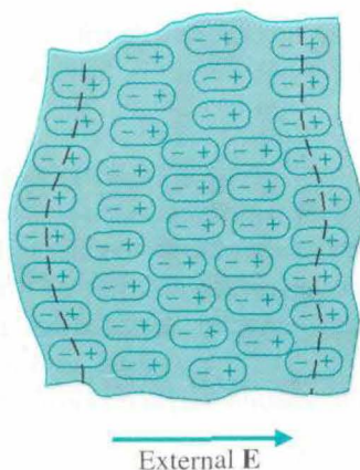
FIGURE 3-14 A cross section of a polarized dielectric medium.
